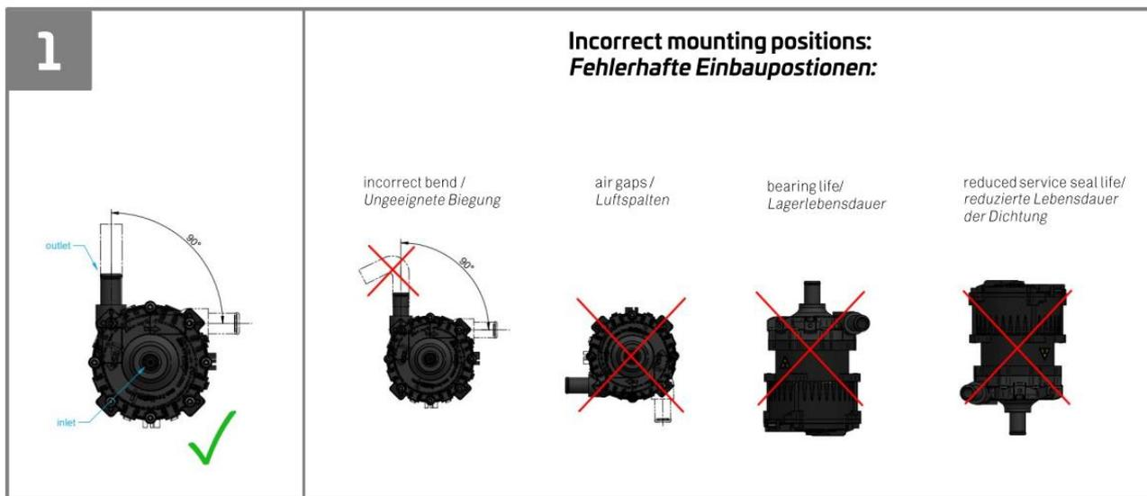
The suction line diameter can not be smaller than the suction port. Smaller dimensions can lead to air entries, followed by problems making the system inefficient and leading to damage on the pump and the whole system. Looking at the pump from the inlet, the pump operates in clockwise direction.
